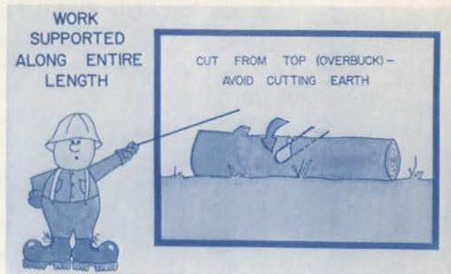
Fig. 11A Use this bucking procedure on work supported along the entire length.
