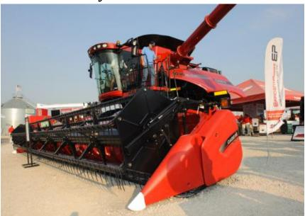
Combines have grown even bigger as now the header alone on a combine can weigh as much as the whole combine did 55 years ago. The header has grown to the average width of 35 to 40-feet long. This gives it the ability to cut double to triple the amount of its ancestors in a single pass. Not to mention, the bulk tank on a combine this big is humongous at 250 bushels.
