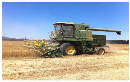
By the early 90s the combine you see above had again outdone the combines of the years before. Its bulk tank was quadruple the size at 120 bushels, compared to the old 40 bushels. The 22-foot header seemed to dwarf the headers of the past that were only 15-foot headers.
