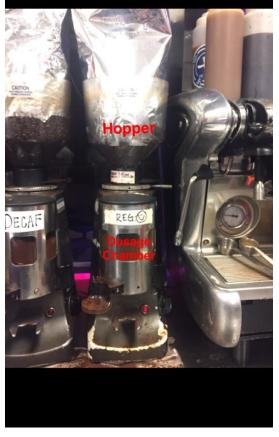
The first thing that you will need is the **grinder.** The grinder is made up of the following parts. The hopper is where the beans are poured before they are ground. The dosage chamber is where the beans fall into after they are ground up.
