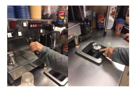
When pulling shots, the first thing you will do is push the porta filter to the left to release it from the espresso machine. Then, you will throw away the old grind that is in the porta filter into the **knock box**.
