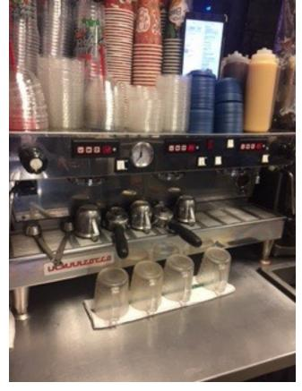
The main component in making coffee is the espresso machine. The main parts of the espresso machine are the porta filters and the steam wands on either side. The buttons above each porta filter are what you push to make the coffee come out.
