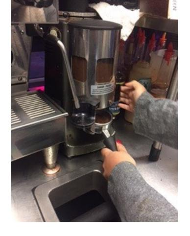
The dosing lever is what releases 7 grams of ground espresso beans per pull. Each drink needs 14 grams though, so you need to pull the lever twice.
