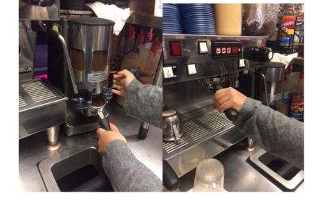
Next you will pull the dosage lever twice and tamp the grounds, like we talked about earlier. Then you will put the porta filter back into the machine and pull it to the right in order to lock it into place.
