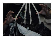
Then begin flaking the nylon fabric layer upon layer according to the line set that each fold is associated
