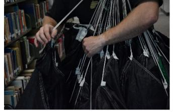
The parachute is actually backwards at this stage so you are working backwards from the tail towards the nose.
