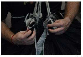
Once you have the slider in place, reach down and pull the tail up over the whole thing like an outer shell.
