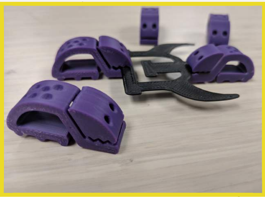
These 3D printed bug clips act as low-pressure clamps for delicate projects in the MILL
