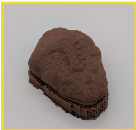
3D printed sandstone sculpture; the file for this model came from the North Carolina Office of State Archaeology
