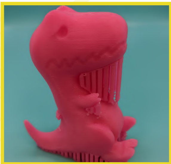
3D printed dinosaur, with support structure
