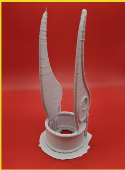
Print with support structure still attached
