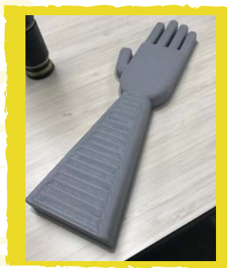
3D printed hand; once sensors are applied, this hand will test the output from a Tesla coil
